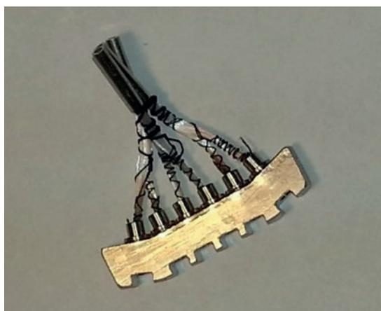
Figure 2. Fiber-optic element of a 3-point sensor
