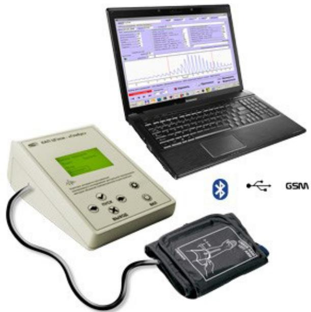
Figure 1. Portable automated hardware & software system for noninvasive examination of central hemodynamics: CH HSS device (Device CH HSS osm GLOBUS).
