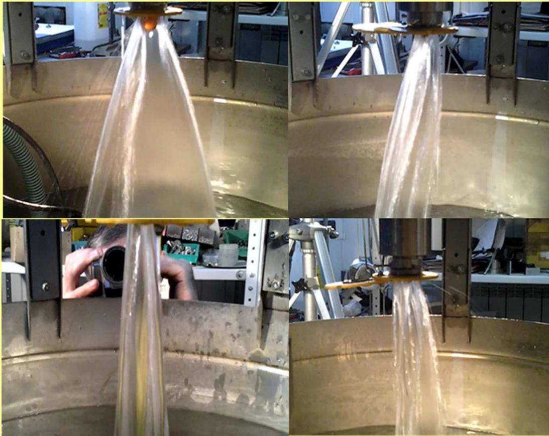
*Figure 4. Destruction of tornado-like jet when flowing over the mechanical aortic valve body: top left: caged ball valve; top right: disc valve MICS; bottom left: bileaflet valve Cardiomed; bottom right: trileaflet valve CorBeat.*
