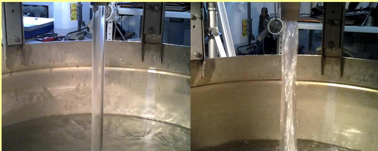
*Figure 3. Glass-like transparent jet stream at outlet of confusor channel without valve inserted (left) vs. jet stream at outlet of the pipe with the same cross-sectional area (right).*
