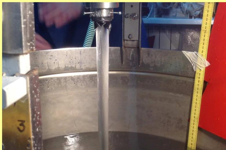
*Figure 5. Maintenance of the tornado-like jet pattern at outlet of confusor channel with cardiac prosthetic device TCV inserted therein.*
